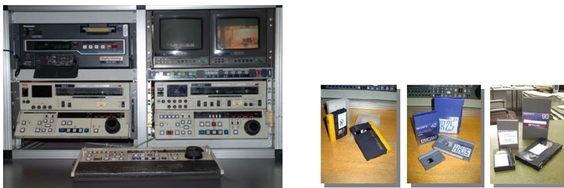
Slika 12: Montažni sklop linearne montaže - Betacam SP, player in recorder, DVCPRO player ter kasete; vir: lasten
