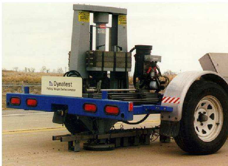
Slika 16: Defletometer s padajočo utežjo (FWD – falling weight deflectometer)
