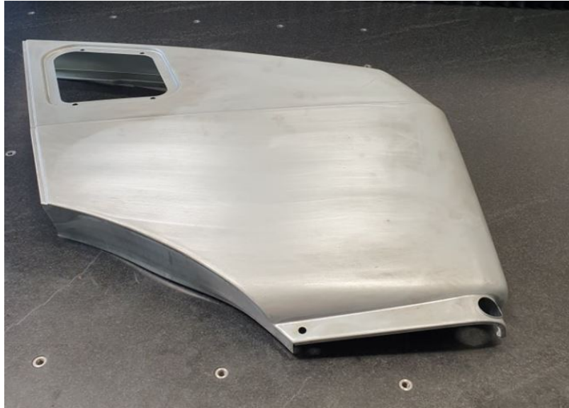
Fig 8 Fender part used as the workpiece in the project.
